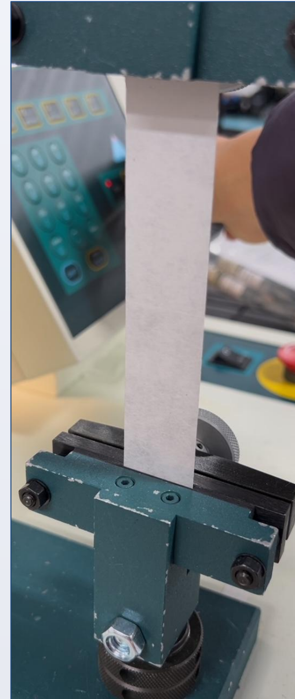
Figure 6. Rectangular paper sample being tested for tensile force in the Tinius Olsen HSK-S Tensile Tester.
