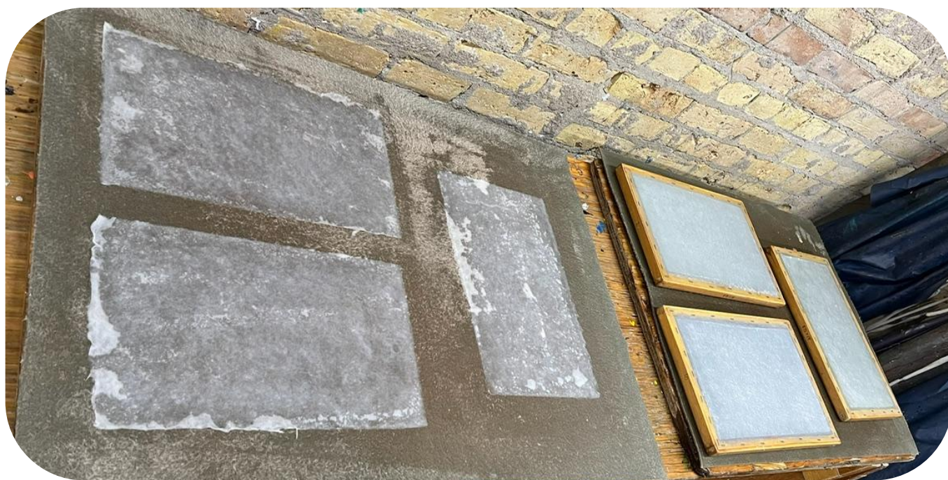
Figure 4. Developed paper sheets on deckles (right) and laid out on a felt (left) (Image courtesy of the researcher).
