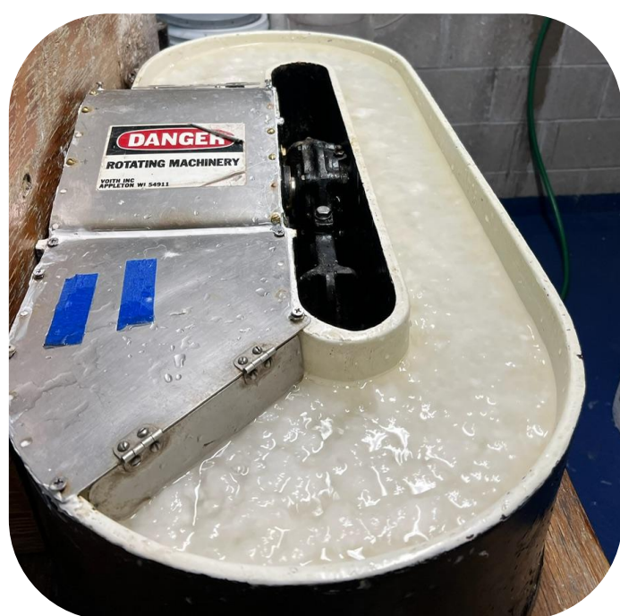
Figure 2. Valley Lab Beater with pulp (Image courtesy of the researcher).
