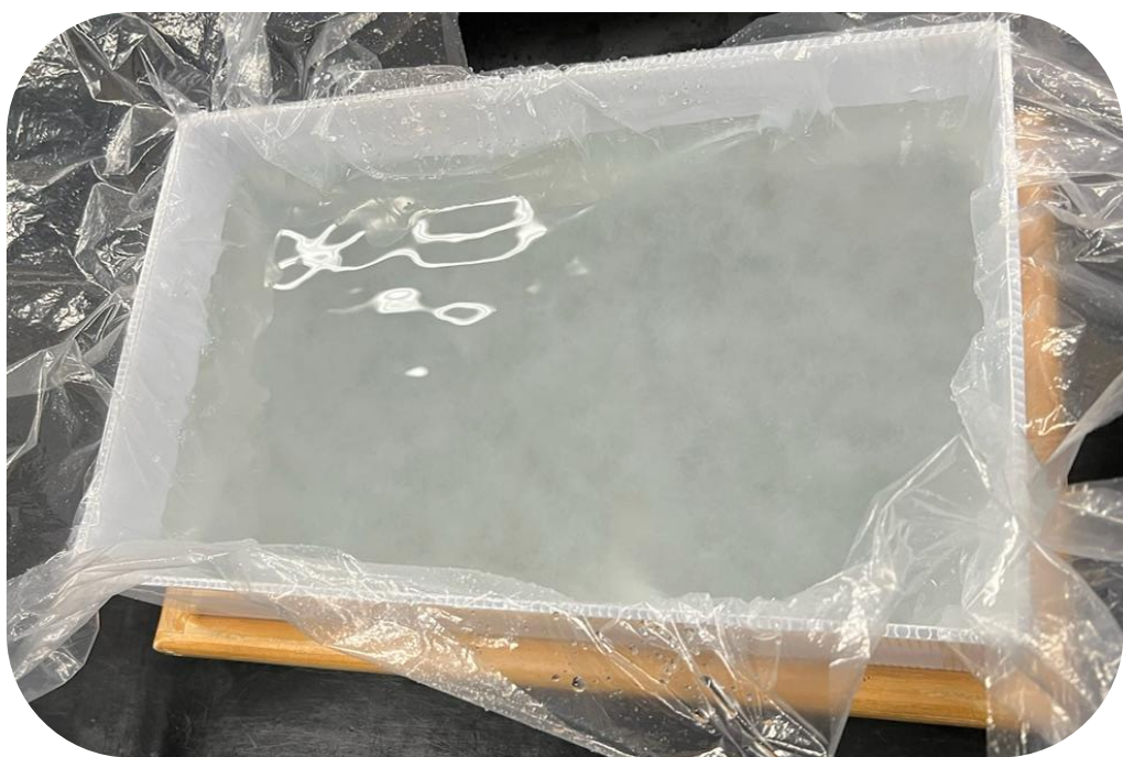
Figure 3. Deckle box filled with pulp (Image courtesy of the researcher).
