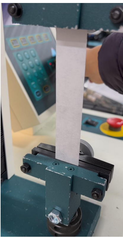
Figure 6. Paper in tensile tester (Image courtesy of the researcher).
