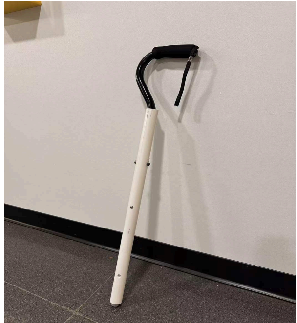
Figure 2: Spring walking sticks with cane handle. The cane handle is used in this mockup, as well as the adjustable feature. There are multiple holes on the PVC tube which allow the extendable tube inside to lock at different holes, thus achieving the desired functionality.
