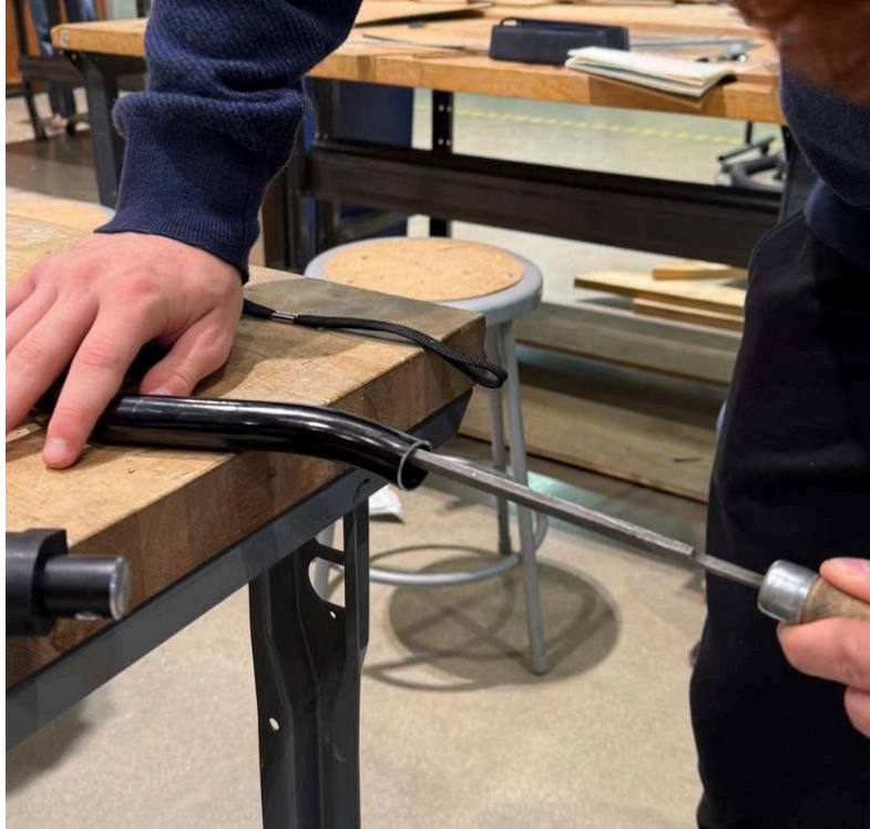
Figure 11: Filing inside of handle
