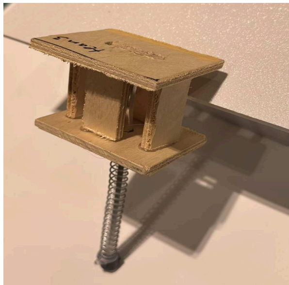
Figure 3: Spring mechanism. The spring mechanism has two states – compressed state and normal state. The compress state locks the spring to stabilize the walking stick, while the normal state allows the spring to function and provide elastic force.
