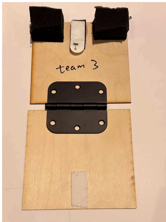
Figure 4: Adjustable spring seat lift. Two cushions are placed at two corners on the “lift” component to provide lifting force. A hinge is used to connect the “seat” and the “lift”
