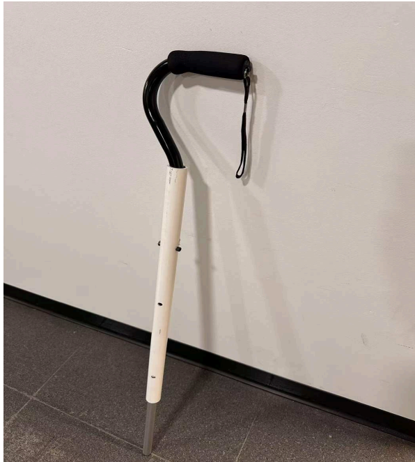
Figure 2: Spring walking sticks with cane handle. The cane handle is used in this mockup, as well as the adjustable feature. There are multiple holes on the PVC tube which allow the extendable tube inside to lock at different holes, thus achieving the desired functionality.
