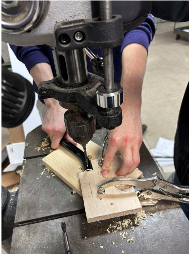
Figure 7: Drilling through the handle
